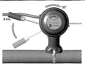
13. Use screwdriver to ratchet on junction box lid. Lid will rotate 30 degrees.
