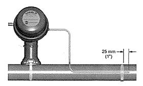
**15.** Fix temperature sensor to pipe using pipe band.
