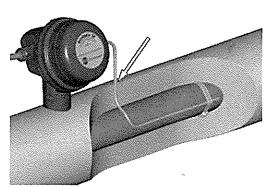
16. Seal temperature sensor penetration through insulation cladding.
