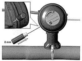
12. Install junction box lid and twist hand tight. Insert screw-driver into ratchet slots located on side of junction box base.
