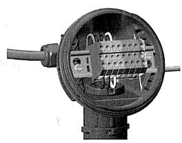
Complete system wiring. Terminal set screws shall be tightened to a torque value of 1.4 Nm (12.4 lb-in). See page 4 for wiring details.
