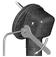
**6** Make sure temperature sensor body is fully inserted into gland connector. Tighten gland connector.
