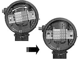
10. Install quick mount terminal blocks and tighten screws (if necessary).
