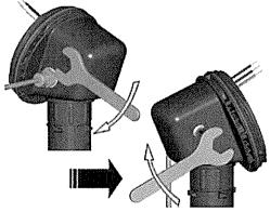
7\_ Install M20 blind plugs in remaining M20 threaded entries.
