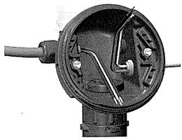
Install control wiring (user supplied, 6 mm² max). 3 wire cable (for 1 sensor) or 6 wire cable (for 2 sensors) with braided earth shield is recommended.
