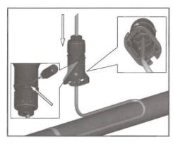
Insert cable into expediter. If mounted on bottom or side of pipe, punch out weep hole.
