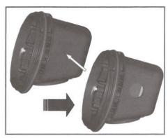
For power connection applications: Use dimple molded into side of junction box base to locate center of hole, drill for user supplied power connection fittings per manufacturer's recommendations.
