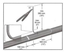
Locate bus connection (HPT and FP only) and cable as shown. Cut end of cable at angle to aid in piercing grommet. Leave additional cable for expansion loop. See page 5 for multiple cable installation tips.
